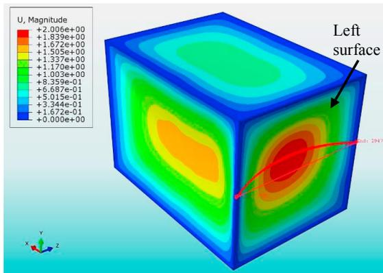
Fig. 7. Warping of the part wall due to rapid internal cooling.
