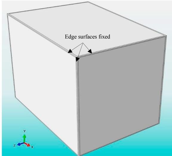
Fig. 3. Fuel tank model with edge surfaces fixed.
