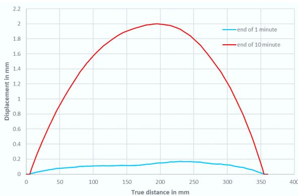
Fig. 8. Nodal displacement values along the horizontal direction (rapid internal cooling).
