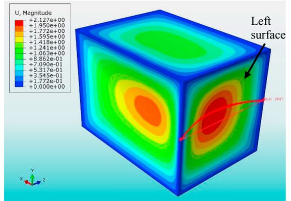
Fig. 5. Warping of the part wall due to rapid external cooling.
