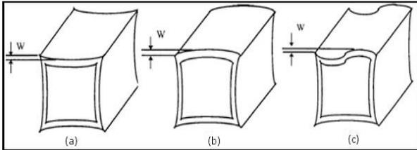
Fig. 1. Types of warpage: a) concave b) convex and c) irregular [5].
