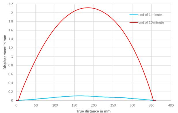
Fig. 6. Nodal displacement values along the horizontal direction (rapid external cooling).
