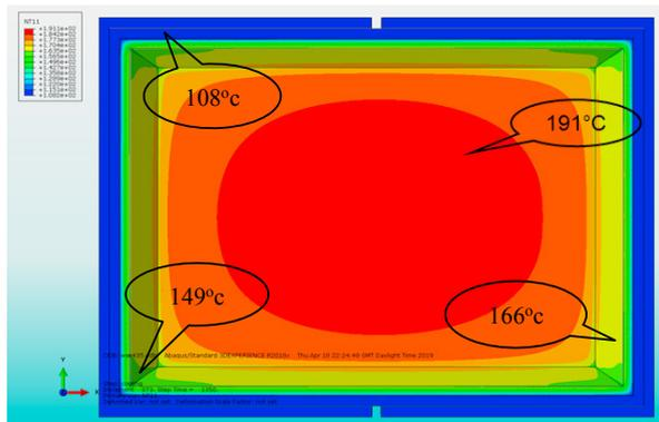
Fig. 4. C/S view of molten polymer stuck against mould wall during cooling cycle (end of 4 minutes).
