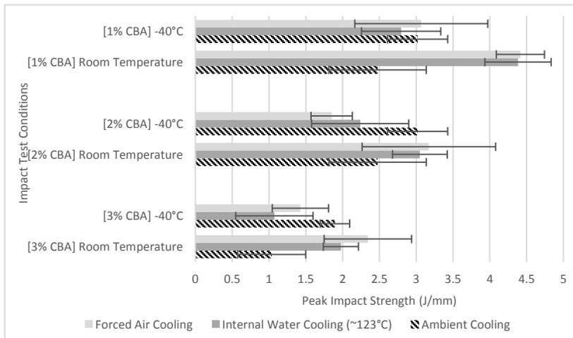
**FIGURE 5.** IS of skin-foam rotationally moulded parts of increasing CBA amount (1%, 2% and 3%) at room temperature and  $-40^{\circ}\text{C}$ .
