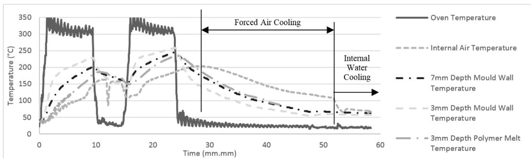
**FIGURE 1.** Internal Water Cooling effects on the Internal Air Temperature of a mould at 195°C for a skin-foam part when internal water spray cooling is applied at 123°C in the cooling cycle.
