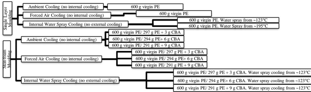
FIGURE 2. Hierarchy of mouldings presented in the current work.
